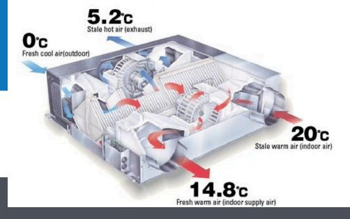
The Lossnay Fresh Air Energy Recovery Systems set a new standard in ventilation by recovering heat from the air inside your office and transferring it to fresh, dry air introduced from outside. Not only providing energy recovery savings in summer by cooling the warmer fresh air to an acceptable level but also providing excellent energy efficiency in winter. Lossnay heat exchangers have a high efficiency thereby eliminating the need for additional electric elements.
